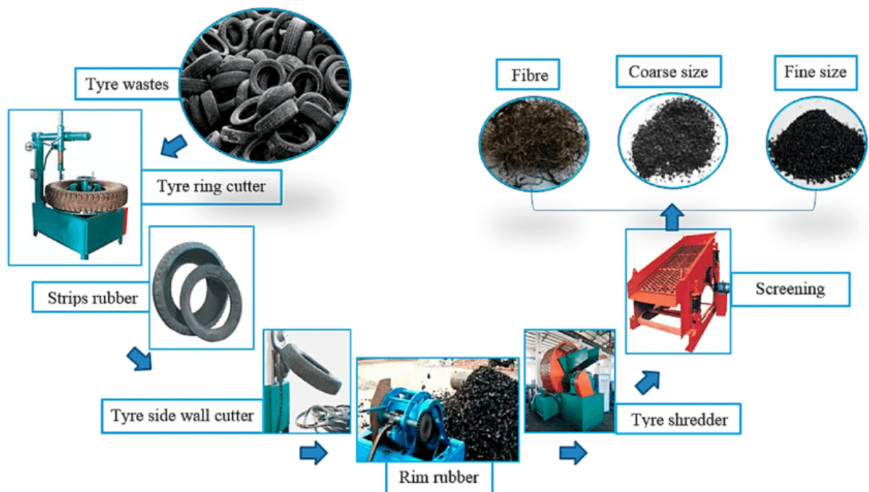
Figure 1: Fine and coarse waste rubber tire crumbs (WRTCs) preparation process (Sources: Mhaya, A.M. et al 2021)
